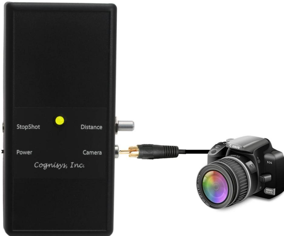
Figure 2 - Stand Alone Connection Diagram
