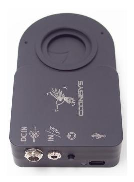
The shutter controller has the following available connections:
