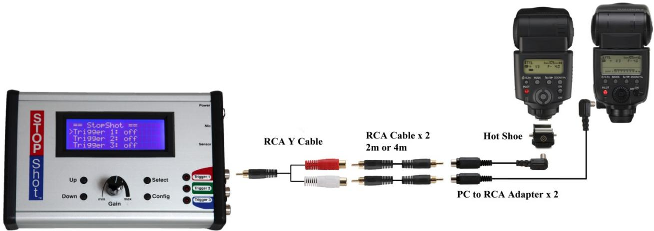
Figure 3 - Connecting two flashes to a single output
