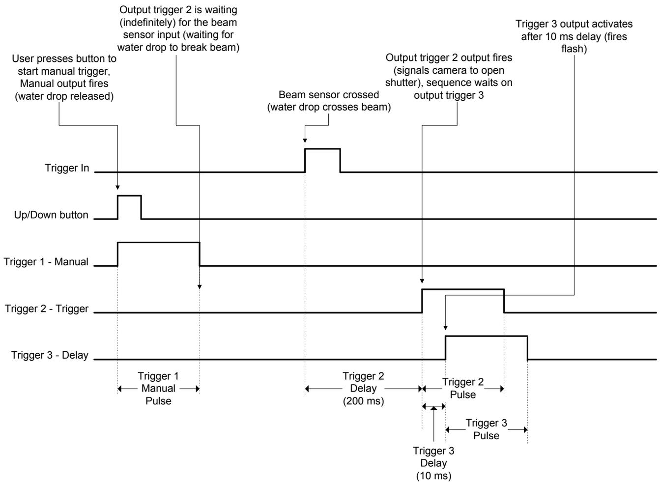
Figure 10 - Sequential Mode Timing Diagram
