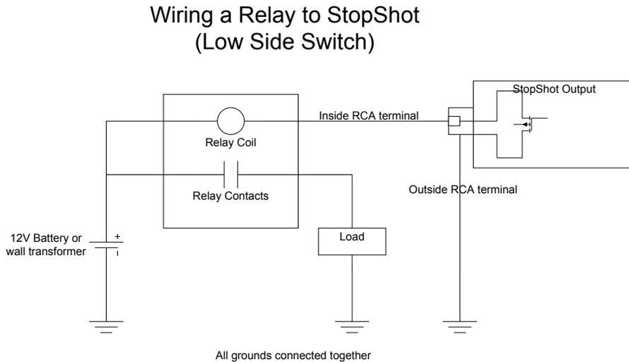
Figure 16 - Wiring an external relay
