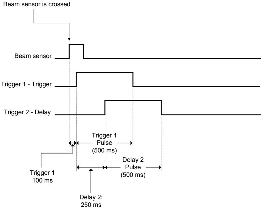
Figure 11 - Delay Synchronization
