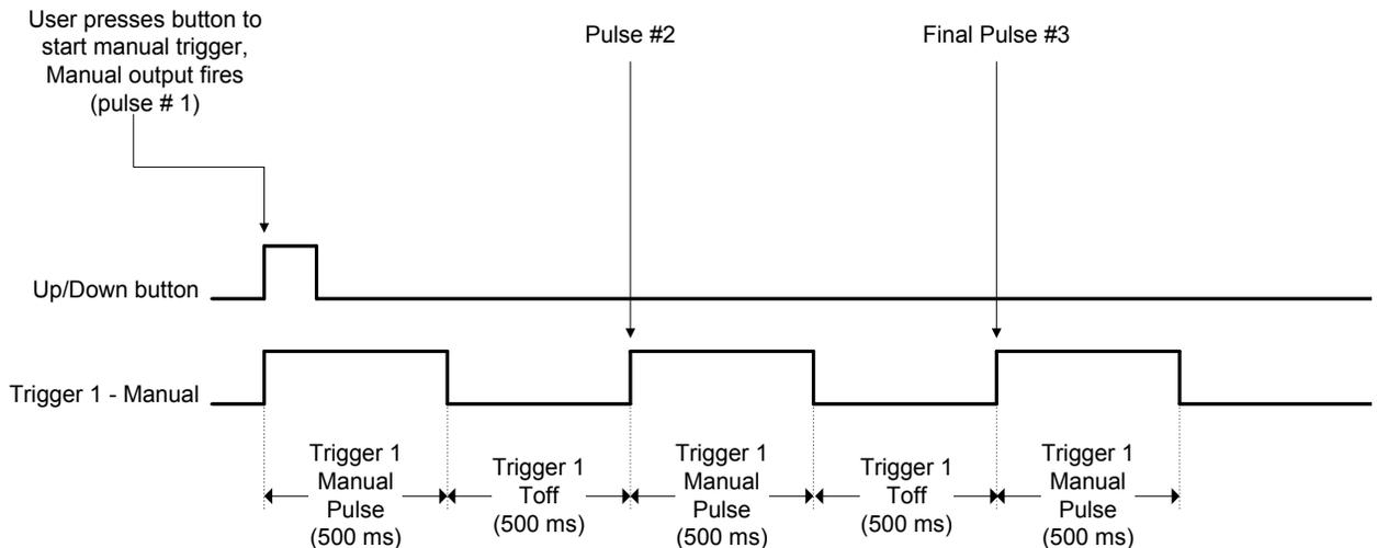
Figure 7 - Manual Mode Timing Diagram
