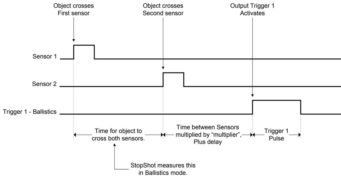
**Figure 9 - Ballistics Timing**
