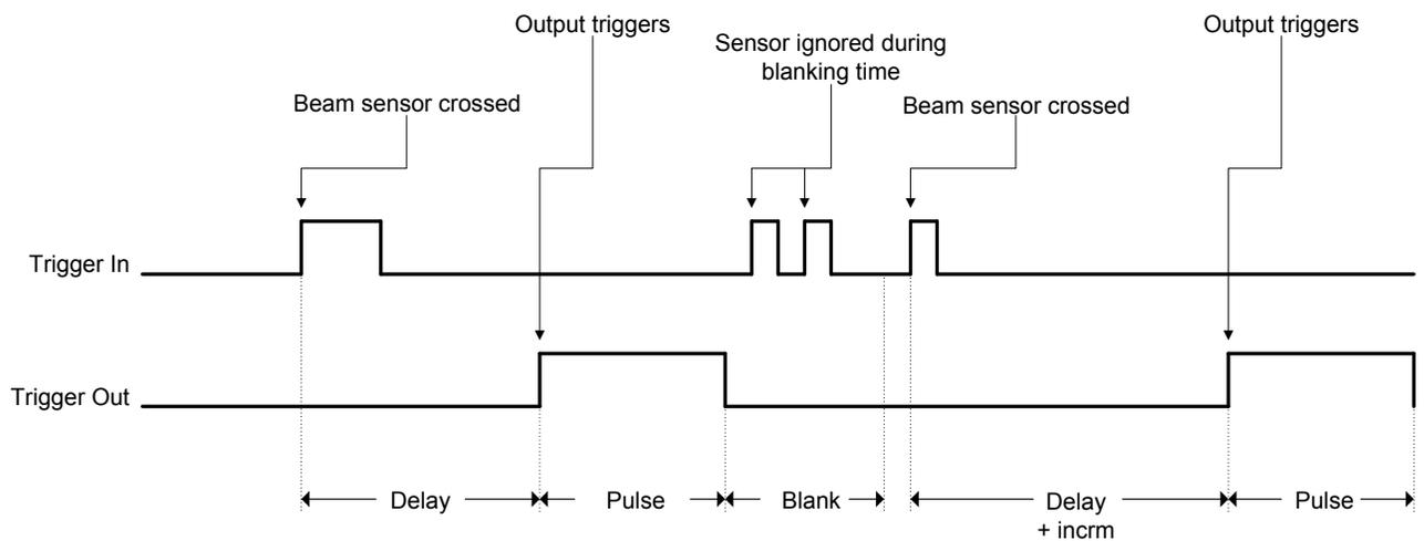
Figure 8 - Trigger Timing Diagram
