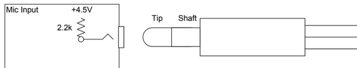
Figure 13 - Microphone Connection
