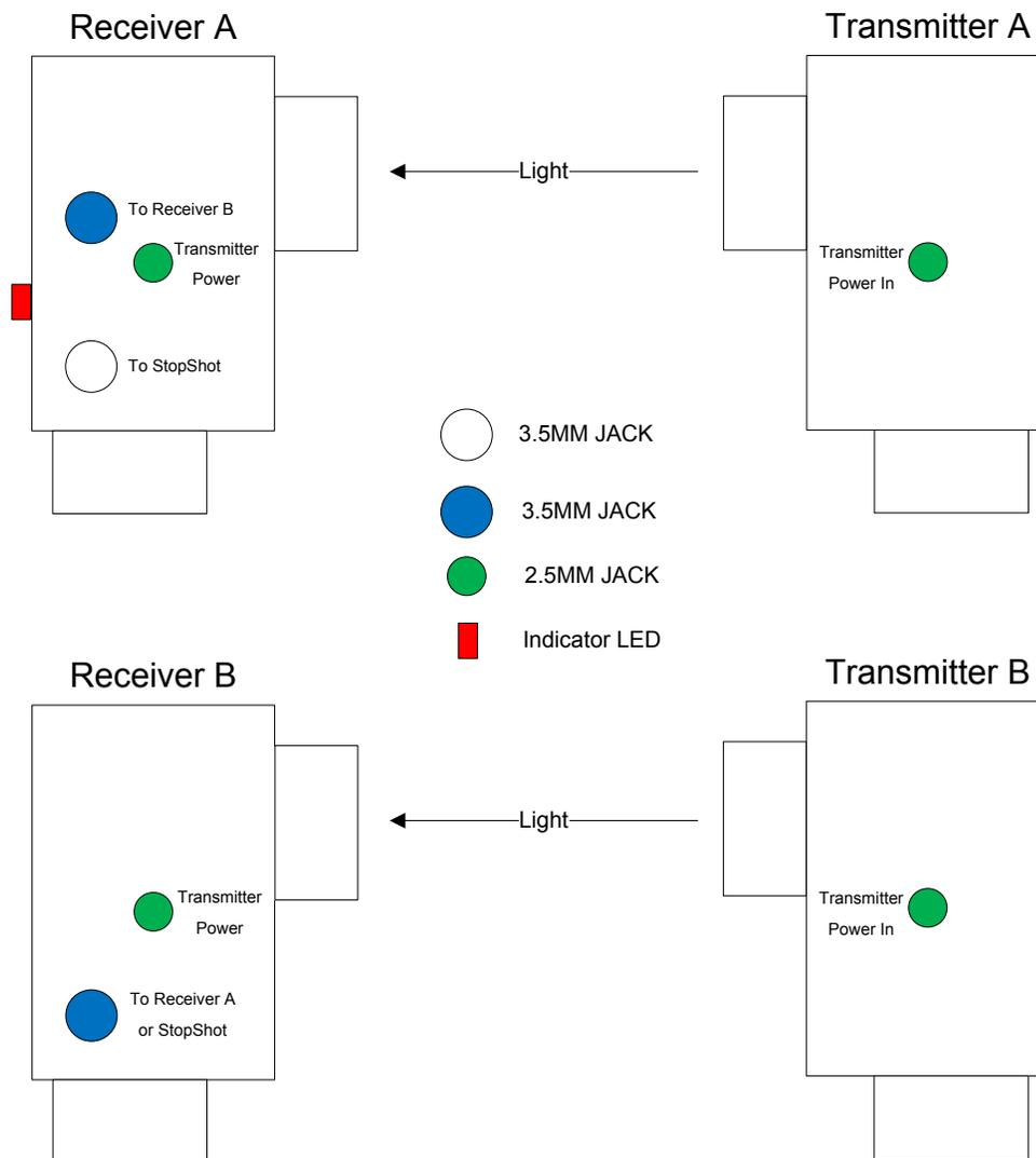
Figure 17 - Cross-beam connections
