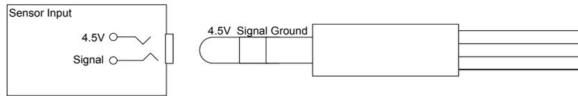
Figure 14 - Sensor Connection
