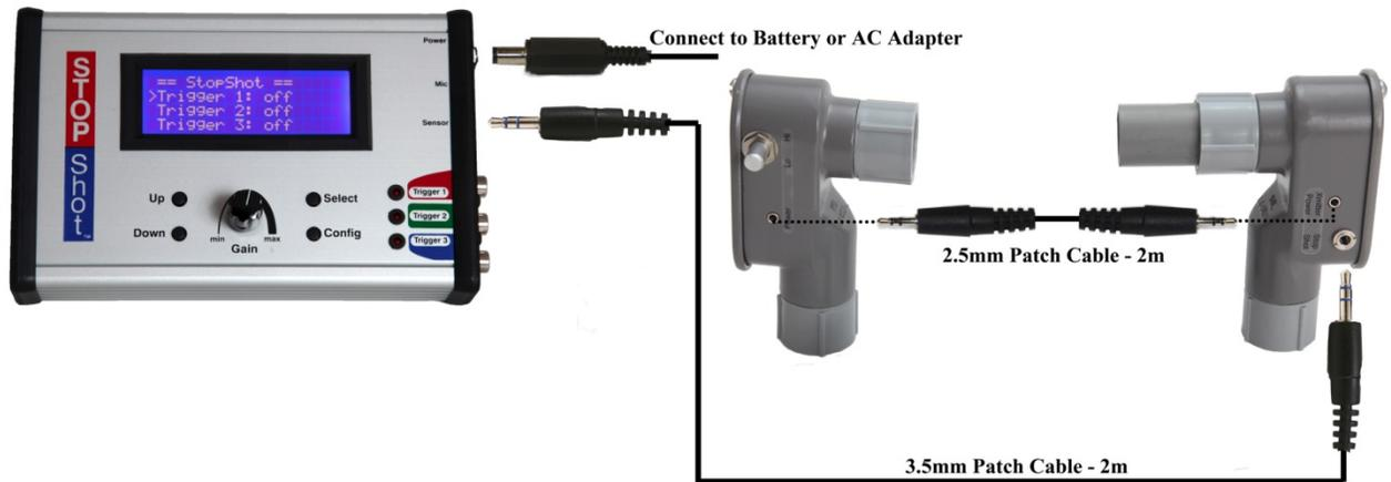
Figure 2 – Connecting the Beam Sensor
