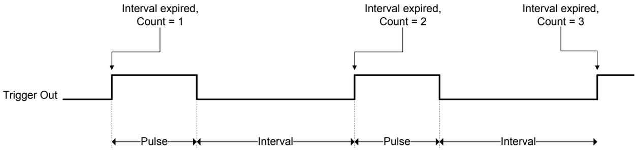
Figure 12 - Time Lapse Timing Diagram
