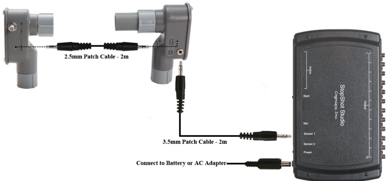
Figure 2 – Connecting the Beam Sensor
