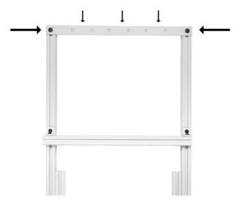
Remove beam sensor screw from bracket on left arm, place sensor bracket as shown, and tighten screw.
