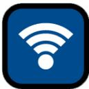
Wifi Button. This turns on and off Wifi. The Blue LED above this button will light when Wifi is enabled. Wifi will automatically turn off after 10 minutes of inactivity to preserve battery life.
