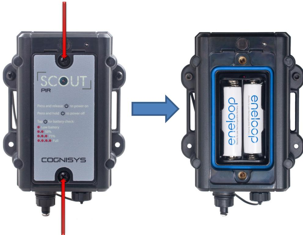
1. Be sure the sensor is clean prior to replacing the batteries otherwise dirt may compromise the weatherproof seal.
